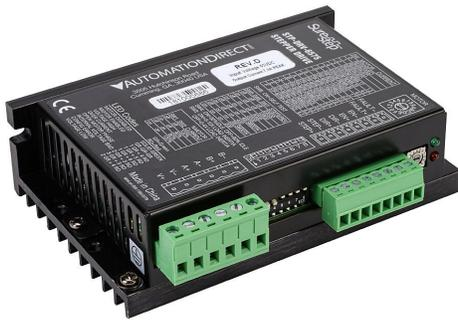
SureStep DC microstepping stepper drive, 7.5A per phase, 2-phase output, 24-75 VDC, bipolar, velocity and position mode, 200 to 20000 steps per revolution.
