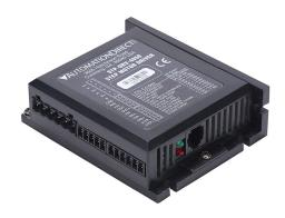
SureStep DC advanced microstepping stepper drive, 5A per phase, 2-phase output, 24-48 VDC, bipolar, velocity and position mode, 200 to 51200 steps per revolution, (1) RS-232 (RJ11) port(s).
