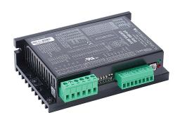
SureStep DC microstepping stepper drive, 4.5A per phase, 2-phase output, 24-48 VDC, bipolar, velocity and position mode, 200 to 20000 steps per revolution.
