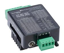
SureStep DC microstepping stepper drive, 3A per phase, 2-phase output, 12-48 VDC, bipolar, velocity and position mode, 200 to 25600 steps per revolution.
