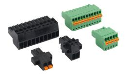
SureStep connector kit, replacement. For use with SureStep STP-MTRD integrated stepper motor/drives except STP-MTRD-17038 and STP-MTRD-17038E. Includes (2) power connectors, (1) RS-485 signal connector and (2) control signal connectors.
