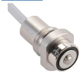
Metrol limit switch, stopper, 10mm diameter, threaded, 1.5mm pitch, 19.8mm length, 2.5mm radius head, stainless steel, 3mm plunger with boot, 1N contact force, (1) N.O. contact(s), 6.5ft/2m cable length, pigtail.
