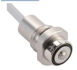
Metrol limit switch, stopper, 10mm diameter, threaded, 1.5mm pitch, 19.8mm length, 2.5mm radius head, stainless steel, 3mm plunger with boot, 1N contact force, N.O. contact(s), 6.5ft/2m cable length, pigtail.
