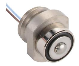
Metrol limit switch, stopper, 10mm diameter, threaded, 1.5mm pitch, 12.8mm length, 2.5mm radius head, stainless steel, 3mm plunger with boot, 1N contact force, (1) N.O. contact(s), 1.6ft/0.5m cable length, core wire.
