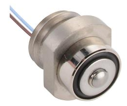
Metrol limit switch, stopper, 10mm diameter, threaded, 1.5mm pitch, 12.8mm length, 2.5mm radius head, stainless steel, 3mm plunger with boot, 1N contact force, N.O. contact(s), 1.6ft/0.5m cable length, core wire.
