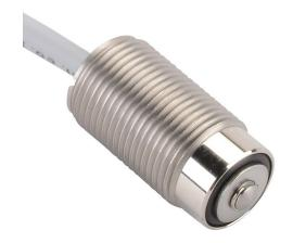
Metrol limit switch, stopper, 10mm diameter, threaded, 0.75mm pitch, 19.8mm length, 2.5mm radius head, stainless steel, 3mm plunger with boot, 1N contact force, N.O. contact(s), 6.5ft/2m cable length, pigtail.
