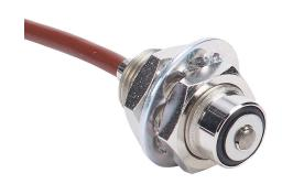
Metrol limit switch, high temperature, stopper, 10mm diameter, threaded, 0.75mm pitch, 19.5mm length, 2.5mm radius head, stainless steel, 3mm plunger with boot, 1N contact force, (1) N.O. contact(s), 6.5ft/2m cable length, pigtail.
