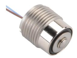
Metrol limit switch, stopper, 10mm diameter, threaded, 0.75mm pitch, 11.8mm length, 2.5mm radius head, stainless steel, 3mm plunger with boot, 1N contact force, N.O. contact(s), 1.6ft/0.5m cable length, core wire.
