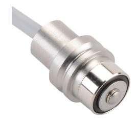
Metrol limit switch, stopper, 11mm diameter, smooth, 18.8mm length, 2.5mm radius head, stainless steel, 3mm plunger with boot, 1N contact force, (1) N.O. contact(s), 6.5ft/2m cable length, pigtail.
