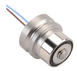
Metrol limit switch, stopper, 11mm diameter, smooth, 11.8mm length, 2.5mm radius head, stainless steel, 3mm plunger with boot, 1N contact force, N.O. contact(s), 1.6ft/0.5m cable length, core wire.
