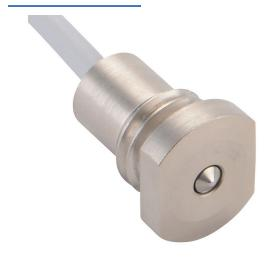
Metrol limit switch, stopper, 10mm diameter, threaded, 1.5mm pitch, 15.5mm length, 13mm flat head, stainless steel, 3mm plunger, 0.8N contact force, (1) N.O. contact(s), 6.5ft/2m cable length, pigtail.
