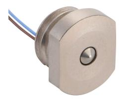
Metrol limit switch, stopper, 10mm diameter, threaded, 1.5mm pitch, 8.5mm length, 13mm flat head, stainless steel, 3mm plunger, 0.8N contact force, (1) N.O. contact(s), 1.6ft/0.5m cable length, core wire.
