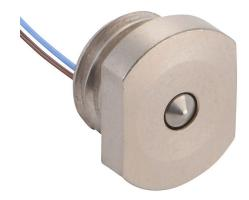
Metrol limit switch, stopper, 10mm diameter, threaded, 1.5mm pitch, 8.5mm length, 13mm flat head, stainless steel, 3mm plunger, 0.8N contact force, N.O. contact(s), 1.6ft/0.5m cable length, core wire.
