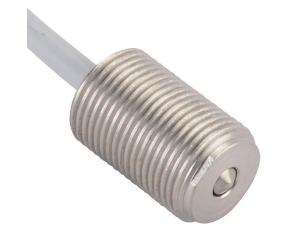
Metrol limit switch, stopper, 10mm diameter, threaded, 0.75mm pitch, 15.5mm length, 8mm flat head, stainless steel, 3mm plunger, 0.8N contact force, (1) N.O. contact(s), 6.5ft/2m cable length, pigtail.
