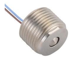
Metrol limit switch, stopper, 10mm diameter, threaded, 0.75mm pitch, 8.5mm length, 8mm flat head, stainless steel, 3mm plunger, 0.8N contact force, (1) N.O. contact(s), 1.6ft/0.5m cable length, core wire.
