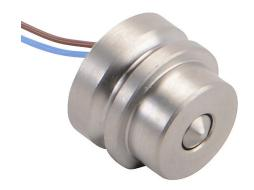
Metrol limit switch, stopper, 10mm diameter, smooth, 8mm length, 8mm flat head, stainless steel, 3mm plunger, 0.8N contact force, (1) N.O. contact(s), 1.6ft/0.5m cable length, core wire.
