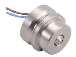
Metrol limit switch, stopper, 10mm diameter, smooth, 8mm length, 8mm flat head, stainless steel, 3mm plunger, 0.8N contact force, N.O. contact(s), 1.6ft/0.5m cable length, core wire.
