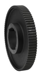
SureMotion timing pulley, cast iron, 3/8in L pitch, 84 tooth, 10.027in pitch diameter, no hub without flanges. For use with 1in wide belt. Requires 2517 series Taper-Lock style bushing.
