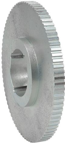
SureMotion timing pulley, cast iron, 3/8in L pitch, 84 tooth, 10.027in pitch diameter, no hub without flanges. For use with 1/2in wide belt. Requires 2517 series Taper-Lock style bushing.
