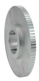
SureMotion timing pulley, cast iron, 3/8in L pitch, 84 tooth, 10.027in pitch diameter, no hub without flanges. For use with 1/2in wide belt. Requires 2517 series Taper-Lock style bushing.
