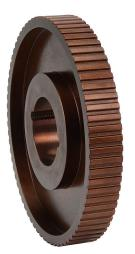
SureMotion timing pulley, cast iron, 3/8in L pitch, 72 tooth, 8.594in pitch diameter, no hub without flanges. For use with 1in wide belt. Requires 2012 series Taper-Lock style bushing.
