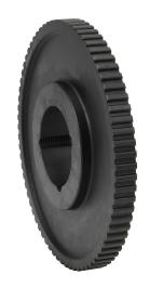
SureMotion timing pulley, cast iron, 3/8in L pitch, 72 tooth, 8.594in pitch diameter, no hub without flanges. For use with 1/2in wide belt. Requires 2012 series Taper-Lock style bushing.
