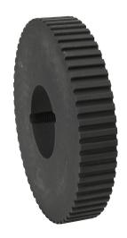
SureMotion timing pulley, cast iron, 3/8in L pitch, 60 tooth, 7.162in pitch diameter, no hub without flanges. For use with 1in wide belt. Requires 2012 series Taper-Lock style bushing.
