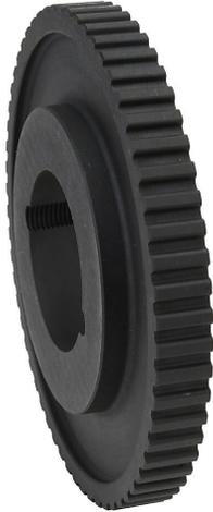
SureMotion timing pulley, cast iron, 3/8in L pitch, 60 tooth, 7.162in pitch diameter, no hub without flanges. For use with 1/2in wide belt. Requires 2012 series Taper-Lock style bushing.
