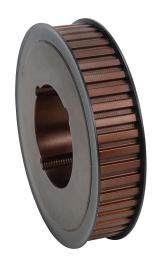
SureMotion timing pulley, ductile iron, 3/8in L pitch, 48 tooth, 5.73in pitch diameter, no hub with flanges. For use with 1in wide belt. Requires 2012 series Taper-Lock style bushing.
