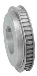
SureMotion timing pulley, ductile iron, 3/8in L pitch, 48 tooth, 5.73in pitch diameter, no hub with flanges. For use with 1/2in wide belt. Requires 2012 series Taper-Lock style bushing.
