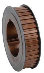
SureMotion timing pulley, ductile iron, 3/8in L pitch, 40 tooth, 4.775in pitch diameter, no hub with flanges. For use with 1in wide belt. Requires 2012 series Taper-Lock style bushing.
