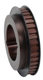
SureMotion timing pulley, ductile iron, 3/8in L pitch, 40 tooth, 4.775in pitch diameter, no hub with flanges. For use with 1/2in wide belt. Requires 2012 series Taper-Lock style bushing.
