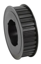
SureMotion timing pulley, ductile iron, 3/8in L pitch, 36 tooth, 4.297in pitch diameter, no hub with flanges. For use with 1in wide belt. Requires 1610 series Taper-Lock style bushing.
