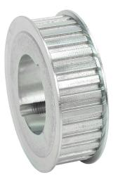
SureMotion timing pulley, ductile iron, 3/8in L pitch, 32 tooth, 3.82in pitch diameter, no hub with flanges. For use with 1in wide belt. Requires 1610 series Taper-Lock style bushing.
