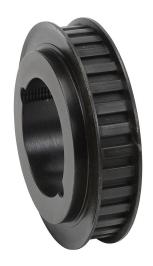
SureMotion timing pulley, ductile iron, 3/8in L pitch, 32 tooth, 3.82in pitch diameter, no hub with flanges. For use with 1/2in wide belt. Requires 1610 series Taper-Lock style bushing.
