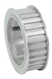
SureMotion timing pulley, ductile iron, 3/8in L pitch, 30 tooth, 3.581in pitch diameter, no hub with flanges. For use with 1in wide belt. Requires 1610 series Taper-Lock style bushing.
