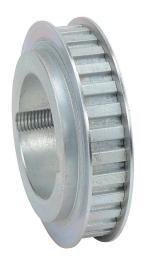
SureMotion timing pulley, ductile iron, 3/8in L pitch, 30 tooth, 3.581in pitch diameter, no hub with flanges. For use with 1/2in wide belt. Requires 1610 series Taper-Lock style bushing.
