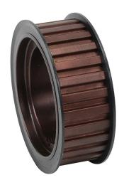
SureMotion timing pulley, ductile iron, 3/8in L pitch, 28 tooth, 3.342in pitch diameter, no hub with flanges. For use with 1in wide belt. Requires 1610 series Taper-Lock style bushing.
