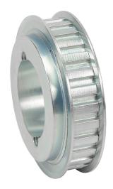
SureMotion timing pulley, ductile iron, 3/8in L pitch, 28 tooth, 3.342in pitch diameter, no hub with flanges. For use with 1/2in wide belt. Requires 1210 series Taper-Lock style bushing.
