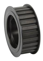
SureMotion timing pulley, steel, 3/8in L pitch, 26 tooth, 3.104in pitch diameter, no hub with flanges. For use with 1in wide belt. Requires 1210 series Taper-Lock style bushing.
