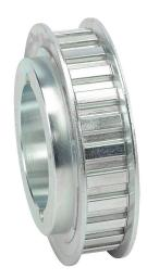
SureMotion timing pulley, steel, 3/8in L pitch, 26 tooth, 3.104in pitch diameter, no hub with flanges. For use with 1/2in wide belt. Requires 1210 series Taper-Lock style bushing.
