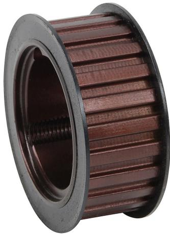
SureMotion timing pulley, steel, 3/8in L pitch, 24 tooth, 2.865in pitch diameter, no hub with flanges. For use with 1in wide belt. Requires 1210 series Taper-Lock style bushing.
