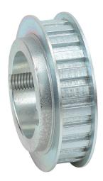
SureMotion timing pulley, steel, 3/8in L pitch, 24 tooth, 2.865in pitch diameter, no hub with flanges. For use with 1/2in wide belt. Requires 1210 series Taper-Lock style bushing.
