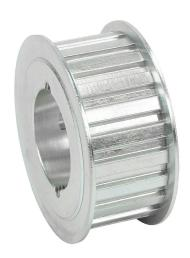
SureMotion timing pulley, steel, 3/8in L pitch, 22 tooth, 2.626in pitch diameter, no hub with flanges. For use with 1in wide belt. Requires 1108 series Taper-Lock style bushing.
