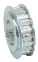
SureMotion timing pulley, steel, 3/8in L pitch, 22 tooth, 2.626in pitch diameter, no hub with flanges. For use with 1/2in wide belt. Requires 1108 series Taper-Lock style bushing.
