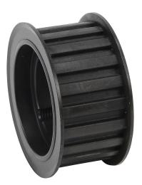
SureMotion timing pulley, steel, 3/8in L pitch, 20 tooth, 2.387in pitch diameter, no hub with flanges. For use with 1in wide belt. Requires 1108 series Taper-Lock style bushing.
