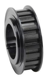
SureMotion timing pulley, steel, 3/8in L pitch, 20 tooth, 2.387in pitch diameter, no hub with flanges. For use with 1/2in wide belt. Requires 1108 series Taper-Lock style bushing.
