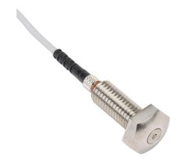
Metrol limit switch, stopper bolt, 10mm diameter, threaded, 1.5mm pitch, 37.5mm length, 4.5mm flat with hex head, stainless steel, 1.5mm plunger, 2N contact force, (1) N.O. contact(s), 6.5ft/2m cable length, pigtail.
