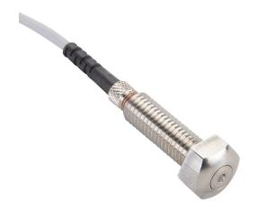
Metrol limit switch, stopper bolt, 8mm diameter, threaded, 1.25mm pitch, 37.5mm length, 4.5mm flat with hex head, stainless steel, 1.5mm plunger, 2N contact force, (1) N.O. contact(s), 6.5ft/2m cable length, pigtail.
