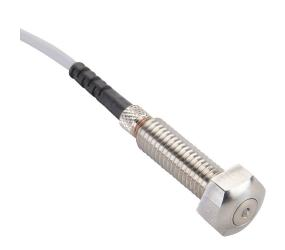
Metrol limit switch, stopper bolt, 8mm diameter, threaded, 1.25mm pitch, 37.5mm length, 4.5mm flat with hex head, stainless steel, 1.5mm plunger, 2N contact force, N.O. contact(s), 6.5ft/2m cable length, pigtail.
