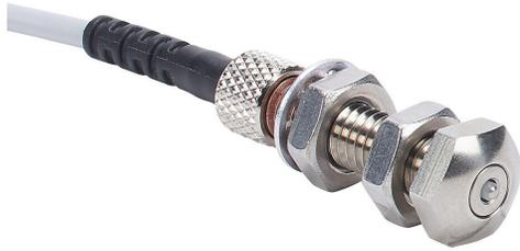
Metrol limit switch, stopper bolt, 6mm diameter, threaded, 1mm pitch, 31.7mm length, 3.4mm flat with hex head, stainless steel, 1.5mm plunger, 2N contact force, (1) N.O. contact(s), 6.5ft/2m cable length, pigtail.
