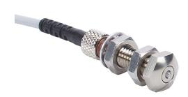
Metrol limit switch, stopper bolt, 6mm diameter, threaded, 1mm pitch, 31.7mm length, 3.4mm flat with hex head, stainless steel, 1.5mm plunger, 2N contact force, N.O. contact(s), 6.5ft/2m cable length, pigtail.
