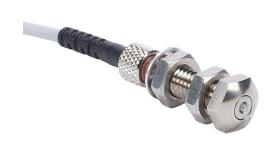
Metrol limit switch, stopper bolt, 6mm diameter, threaded, 1mm pitch, 31.7mm length, 3.4mm flat with hex head, stainless steel, 1.5mm plunger, 2N contact force, (1) N.O. contact(s), 6.5ft/2m cable length, pigtail.
