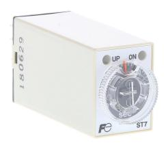
Fuji Electric on-delay relay timer, 4 to 60 seconds selectable timing range, 24 VDC operating voltage, 3A contact rating, (1) DPDT timed relay output(s), socket mount, 8-pin. Requires Fuji Electric TP88X2 timer socket.
