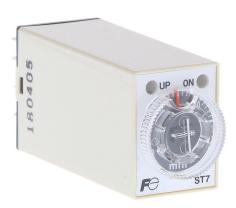
Fuji Electric on-delay relay timer, 4 to 60 minutes selectable timing range, 24 VDC operating voltage, 3A contact rating, (1) DPDT timed relay output(s), socket mount, 8-pin. Requires Fuji Electric TP88X2 timer socket.
