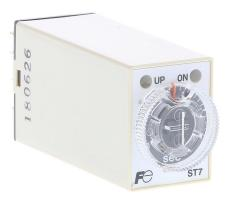
Fuji Electric on-delay relay timer, 0.4 to 5 seconds selectable timing range, 24 VDC operating voltage, 3A contact rating, (1) DPDT timed relay output(s), socket mount, 8-pin. Requires Fuji Electric TP88X2 timer socket.
