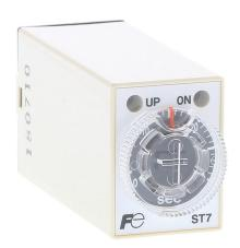
Fuji Electric on-delay relay timer, 2 to 30 seconds selectable timing range, 24 VDC operating voltage, 3A contact rating, (1) DPDT timed relay output(s), socket mount, 8-pin. Requires Fuji Electric TP88X2 timer socket.
