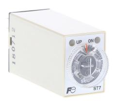
Fuji Electric on-delay relay timer, 4 to 60 seconds selectable timing range, 100-120 VAC operating voltage, 3A contact rating, (1) DPDT timed relay output(s), socket mount, 8-pin. Requires Fuji Electric TP88X2 timer socket.
